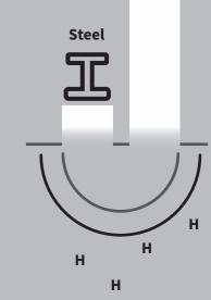
Because of these properties of gold regarding hydrogen permeability, STS gold-coated stainless membranes as standard for hydrogen applications.
